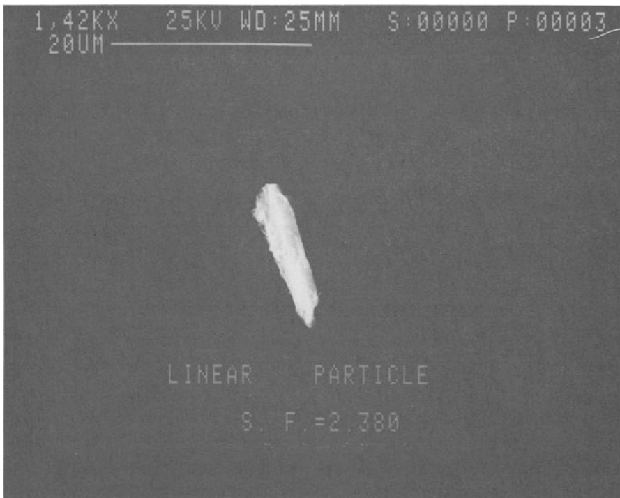
FIG. 1— SEM image of an irregular particle shown with the PRC program's calculated shape factor. Magnification: \times 1717 .
